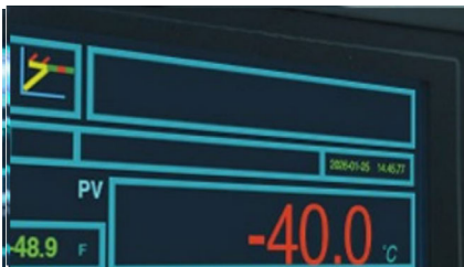
HMI Display: Low-Temperature Performance Test Under -40°C
