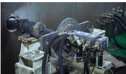
Hydraulic Pump: Low-Temperature Performance Test Under -40°C
