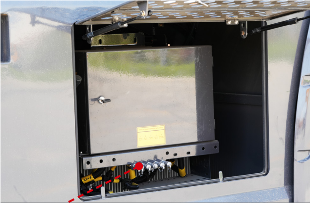
The pressure testing ports are centrally arranged.
