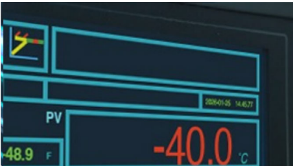
HMI DISPLAY: LOW-TEMPERATURE PERFORMANCE TEST UNDER -40° C
