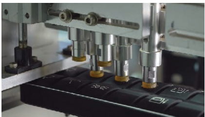
PANEL BUTTONS: CYCLED 12 MILLION TIMES
