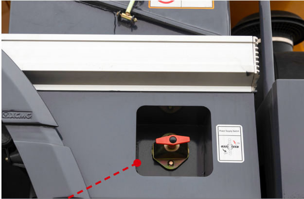
Main power switch
