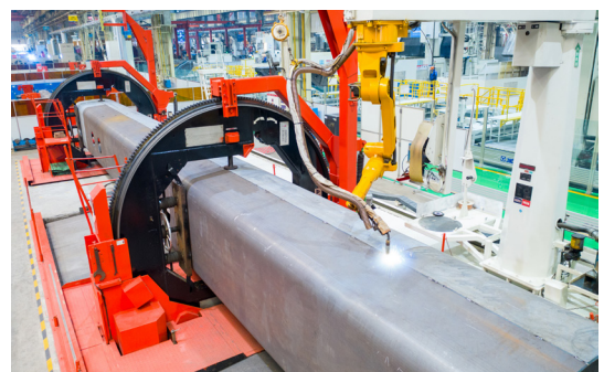
UNMANNED AUTOMATIC WELDING
