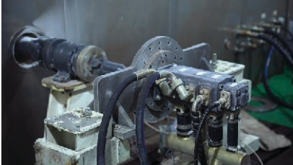
HYDRAULIC PUMP: LOW-TEMPERATURE PERFORMANCE TEST UNDER -40° C
