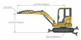
1. The lifting capacity ratings are based on ISO10567.
