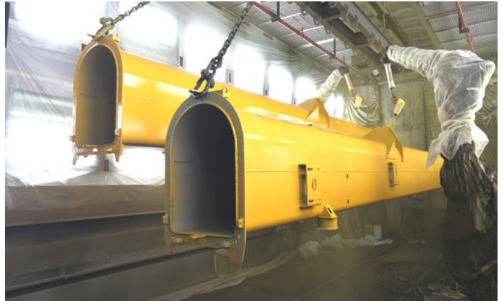
Automated Painting to Ensure Consistent Quality
