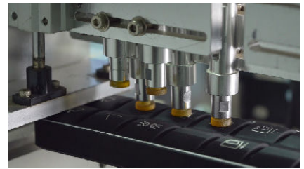
Panel Buttons: Cycled 12 Million Times
