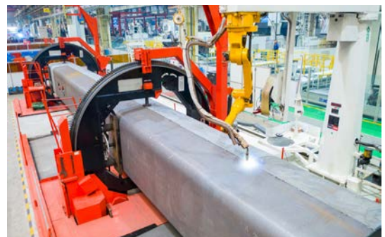
UNMANNED AUTOMATIC WELDING
