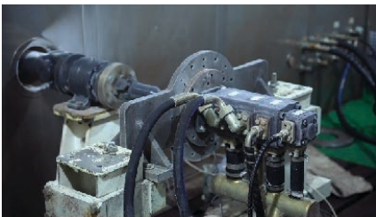
Hydraulic Pump: Low-Temperature Performance Test Under -40 °C
