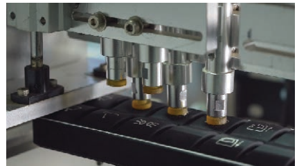
Panel Buttons: Cycled 12 Million Times
