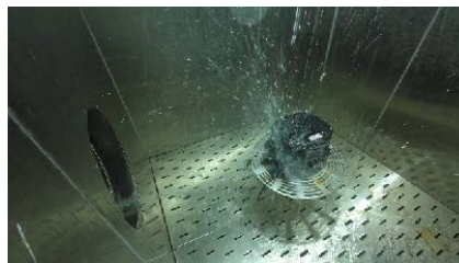
LENGTH MEASUREMENT SENSOR: 48-HOUR RAIN TEST
