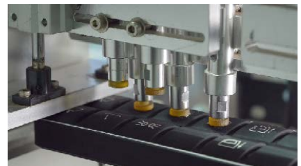
PANEL BUTTONS: CYCLED 12 MILLION TIMES
