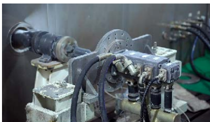
HYDRAULIC PUMP: LOW-TEMPERATURE PERFORMANCE TEST UNDER -40°C
