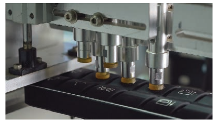
Panel Buttons: Cycled 1.2 Million Times
