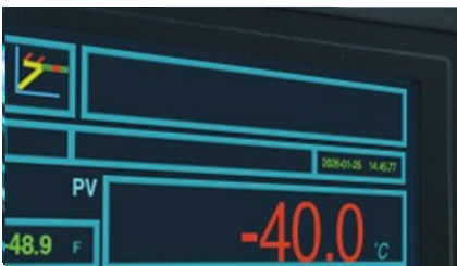
HMI Display: Low-Temperature Performance Test Under -40 °F
