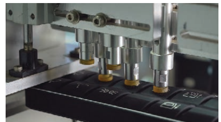
Panel Buttons: Cycled 12 Million Times
