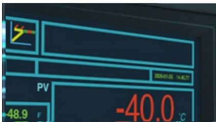
HMI DISPLAY: LOW-TEMPERATURE PERFORMANCE TEST UNDER -40°C
