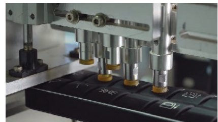
PANEL BUTTONS: CYCLED 12 MILLION TIMES
