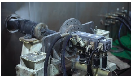
Hydraulic Pump: Low-Temperature Performance Test Under -40 C
