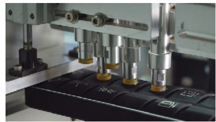
Panel Buttons: Cycled 12 Million Times
